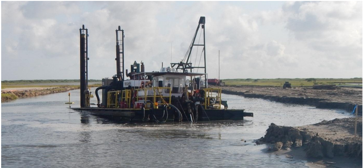
Figure 1. Hydraulic dredge working in Cedar Bayou.
